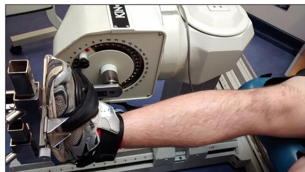
**Figure 3** — Isokinetic dynamometer setup for assessment of passive muscle tension and maximal voluntary contraction. Ankle flexed at 90° relative to the tibia.
