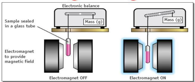
Paramagnetic: substance is attracted to a magnetic field. Substance has unpaired electrons.
